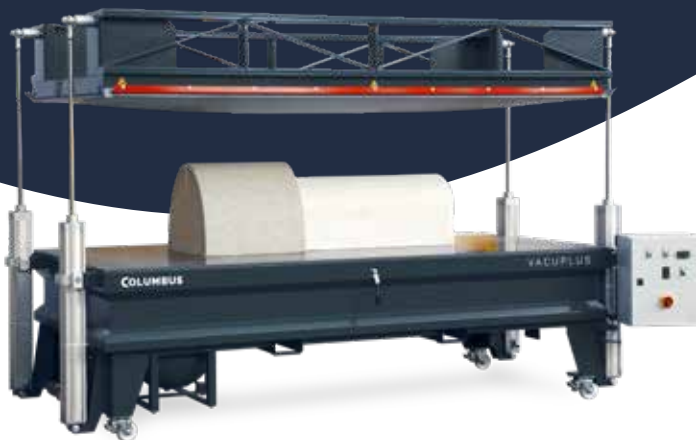
Vacuplus with vertical opening mechanism, digital vacuum pressure controller and 200 l tank
